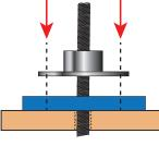
**CORRECT** - Hole drilled 1/2" larger than Rod diameter and equal pressure is applied to fully seat CNX on the BPW.
