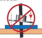
**INCORRECT** - Over-sized hole, Rod exceeds tolerance for plumb.
